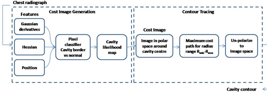
Fig. 1. Proposed cavity contour segmentation approach
