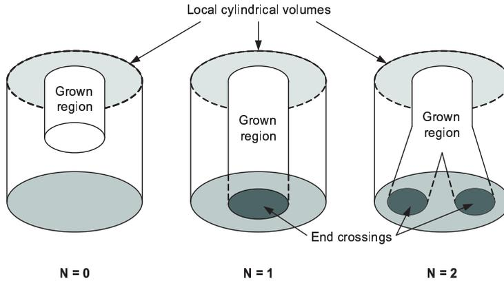
**Fig. 1.** Illustration of different number of end crossings ( $N$ ). A view looking up at the cylinders is shown. The number of end crossings determines how the algorithm will proceed in the next iteration.
