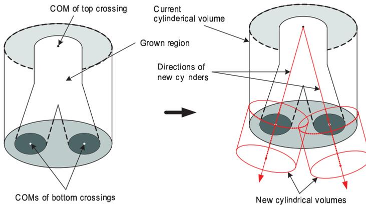
**Fig. 2.** Illustration of new cylindrical volume construction ( $N=2$ ). A view looking up at the cylinders is shown. The left figure shows the current cylindrical volume, and the right figure shows both current and new cylindrical volume. The directions of the new cylindrical volumes are determined by connecting the center of masses of crossings.
