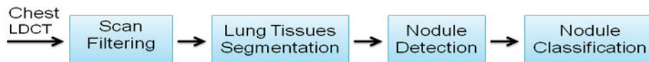
Fig. 1: A block diagram of the major steps involved in computer-based analysis of LDCT of the chest in order to detect and classify doubtful lung nodules.
